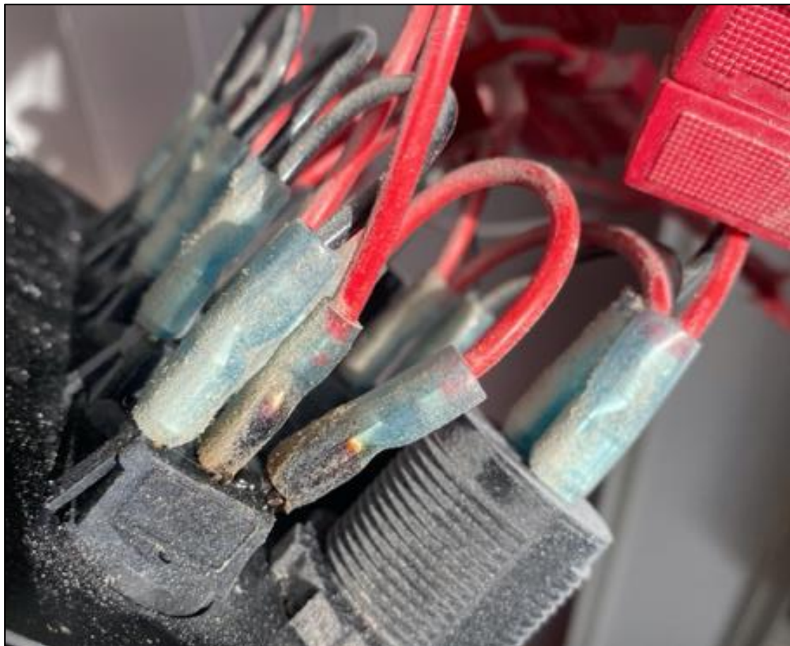
Photograph 16 – Evidence of high resistance/excessive heat to water pump switch
